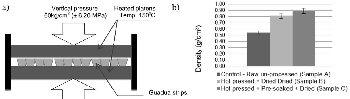
Figure 44. (a) Diagram of the densification process (b) Graph of the oven dry density of Samples A, B, and C.
