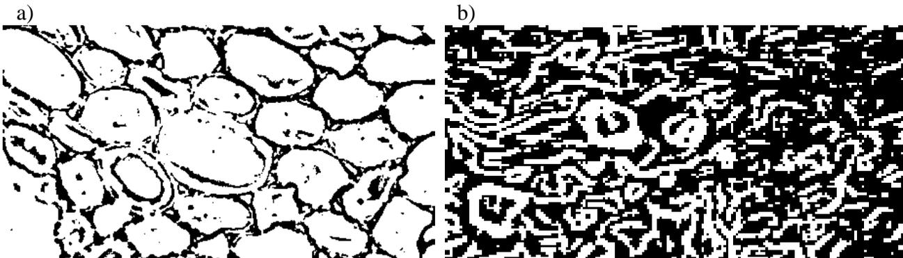
Figure 7. Digitally contrasted pictures from two inverted reflected-light microscope images of the same region before (a) and after (b) densification.
