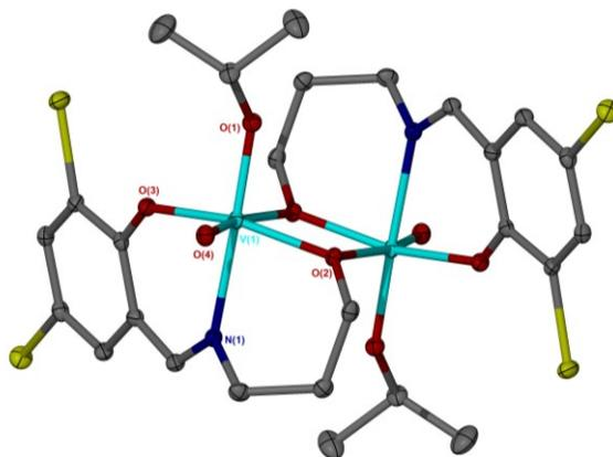
**Figure 4:** Solid state structure of VO(2)(O<sup>i</sup>Pr) ellipsoids are shown at the 30% probability level and hydrogen atoms have been removed for clarity.
