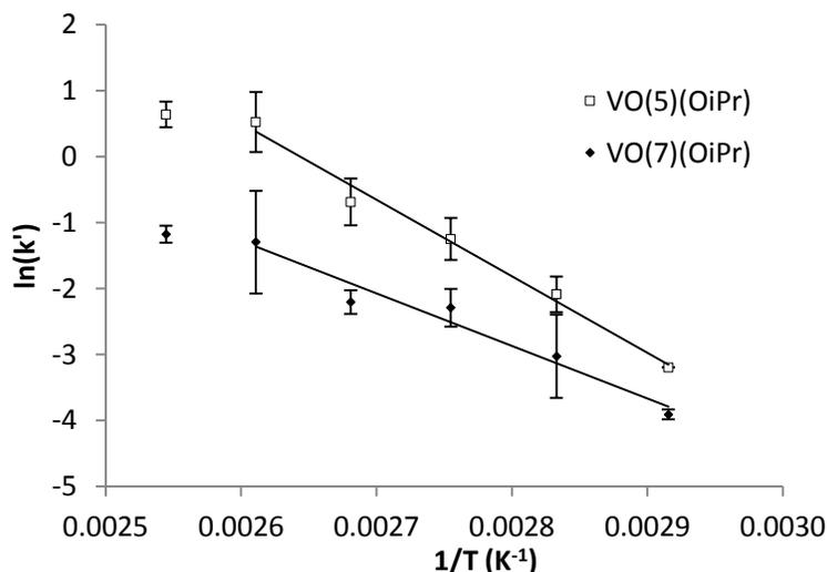
**Figure 8:** Arrhenius plots for the degradation of 2-phenoxy-1-phenylethanol by VO(5,7)(O<sup>i</sup>Pr).
