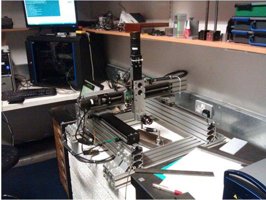
Figure 1 - Picture of the 3 axis machine performing a ball-bar test
