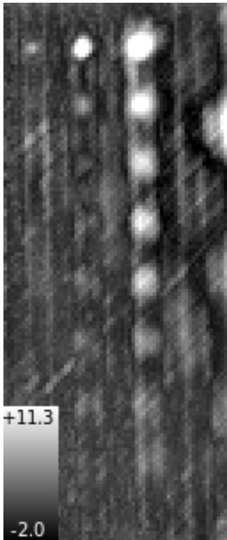
Figure 13: Fused image obtained from the extracted FMTWI phase images at the five analysis frequencies.
