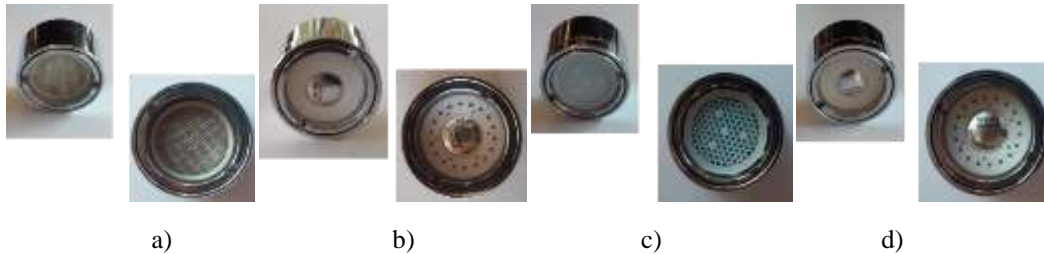
142 a) b) c) d) 143 Fig. 2. Characteristics of the different aerators: a) aerator A (aerated flow; Q = 4.7 l/min); b) aerator B (spray 144 flow; Q = 3.9 l/min); c) aerator C (aerated flow; Q = 3.4 l/min); d) aerator D (spray flow; Q = 2.0 l/min) 145
