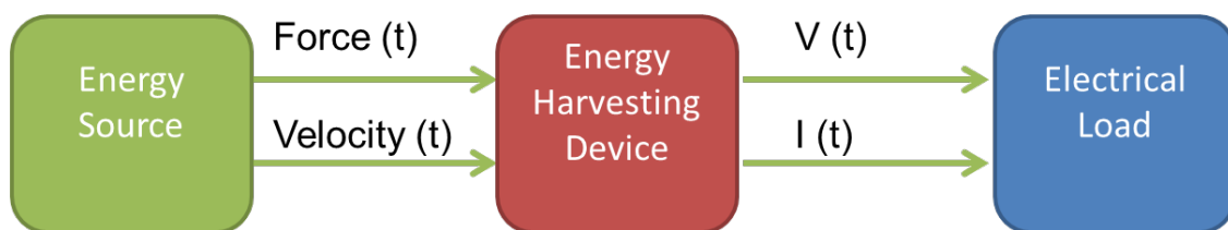
Figure 2: Schematic diagram of an energy harvesting system
