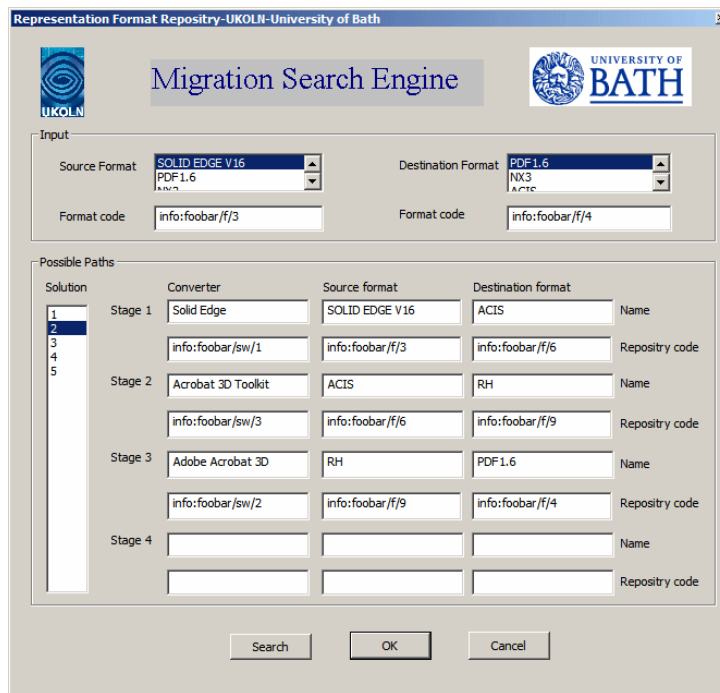
Figure 3 – The query interface for searching for migration paths between two formats, allowing a maximum of four migration stages.
