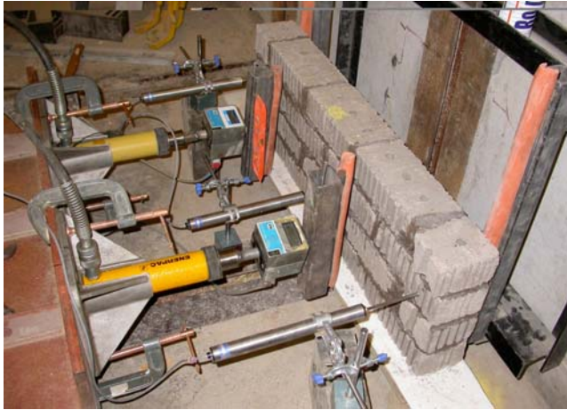
Figure 8. Set-up for flexural tests (perpendicular to bed joint) according to BS EN 1052-2:1999 (BSI, 1999b)
