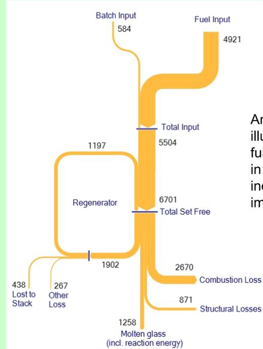
An exergy analysis, such as that illustrated here, for a glass furnace, showing flows of exergy in MJ per tonne of output, can indicate areas of a process where improvement is possible.
