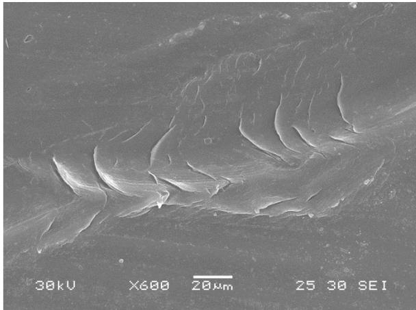
**Figure 2: Smearing of Gear Flanks  $6 \times 10^6$  Cycles**
