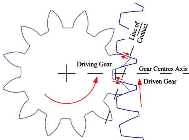
Figure 1: Gear Contact and Sliding
