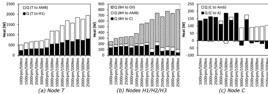
**Figure 5: Predicted heat flows in selected turbocharger nodes**
