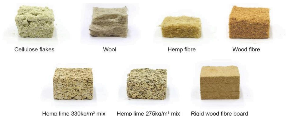
Figure 1: Insulation specimens.
