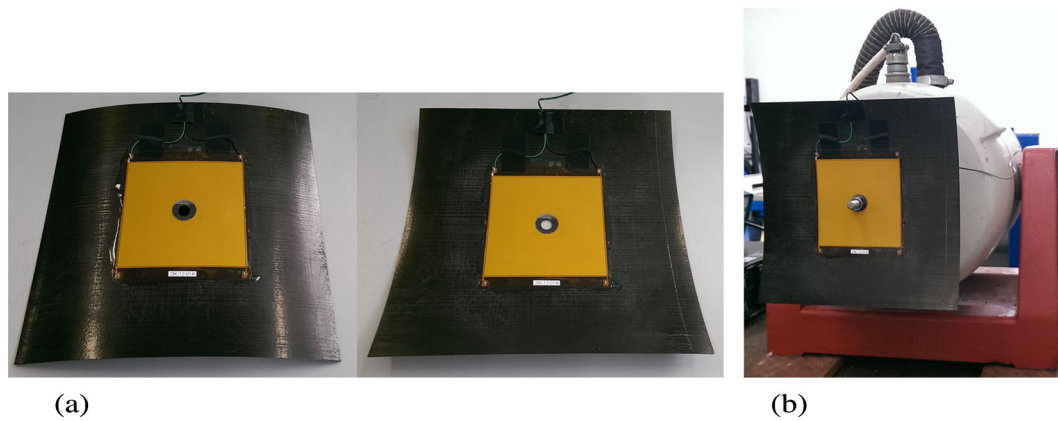
Fig. 1. (a) Stable shapes of a 190 mm \times 190 mm [0/90]_T bistable laminate plate, and (b) experimental setup showing mechanical shaker attachment. A square CFPR laminate is coupled to smaller square piezoelement (MFC, Micro-Fibre-Composite) but the output voltage is not measured in this experiment.
