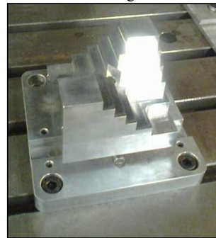
Fig.6: Initial Artefact used for 3-Axis Probing
