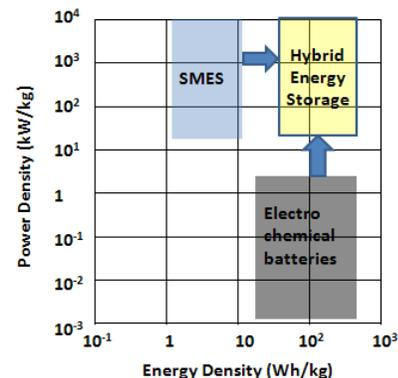
Fig.1 The configuration of Hybrid Energy Storage System
