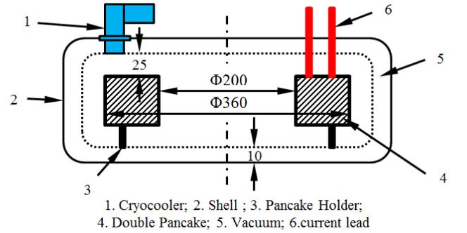
Fig. 5 Schematic of cooling and thermal insulation system
