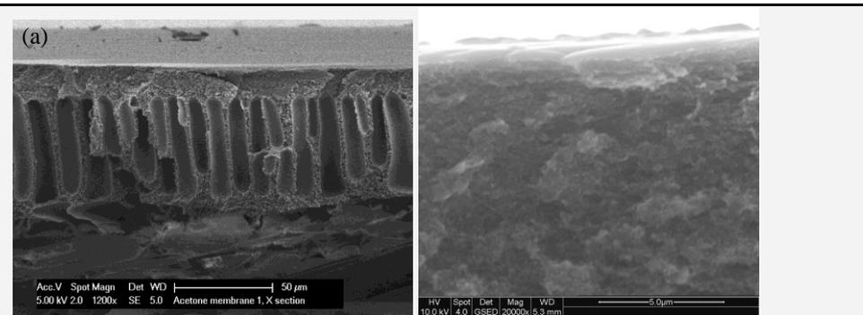
Figure 1: Membrane (25wt% P84 + 65wt% NMP+ 10wt% acetone, 60s evaporation time) imaged (a) dry by SEM, and (b) wetted after soaking in ethanol in the ESEM, where a more gelatinous microstructure is revealed.
