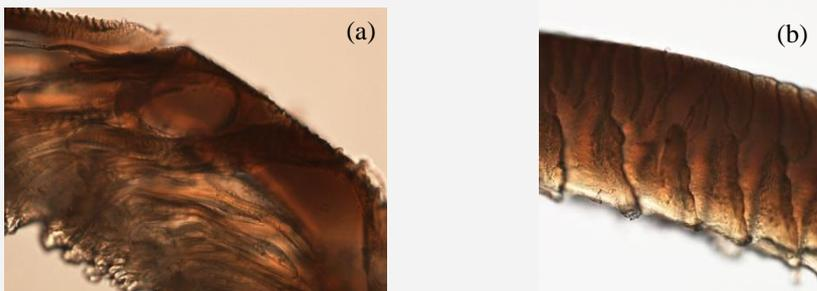
Figure 2: Imaging by DIC microscopy in acetone, showing the difference between evaporation times in the microstructure. Both membranes are from 25 wt% P84, 75wt% NMP, with evaporations: (a) 0 sec, (b) 60 sec.
