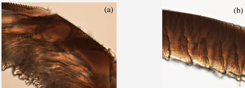
Figure 2: Imaging by DIC microscopy in acetone, showing the difference between evaporation times in the microstructure. Both membranes are from 25 wt% P84, 75wt% NMP, with evaporations: (a) 0 sec, (b) 60 sec.
