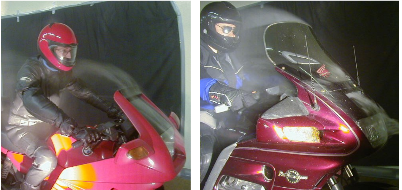
Figure 3: Flow over the windscreen of two different touring motorcycles: BMW K1100, left; Honda ST1100, right.
