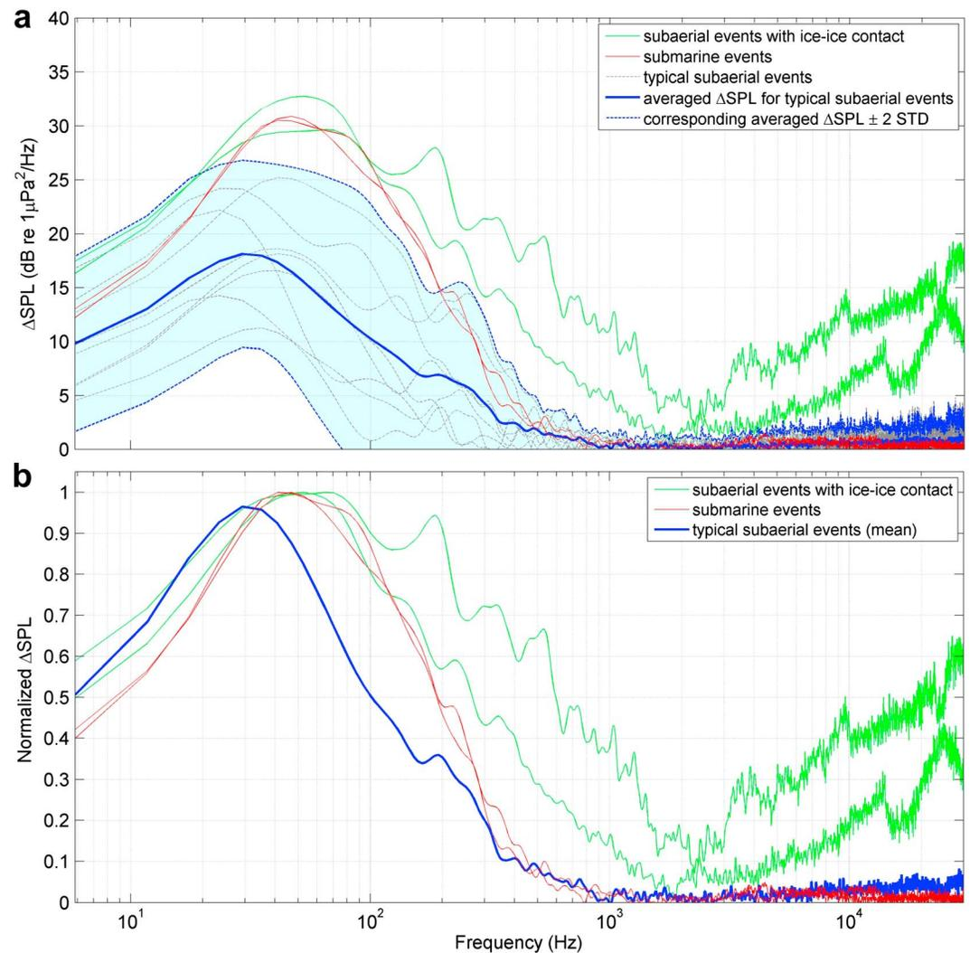
**Figure 2.** Time-averaged sound pressure levels (SPLs), both (a) before and (b) after normalization by their maximum values, during the 12 selected calving events, smoothed and with no significant background noise. For typical subaerial detachments, event-averaged nonnormalized  $\Delta$ SPL is shown with  $\pm 2$  standard deviations (the smaller number of events in the other modes precluded the use of standard deviations).
