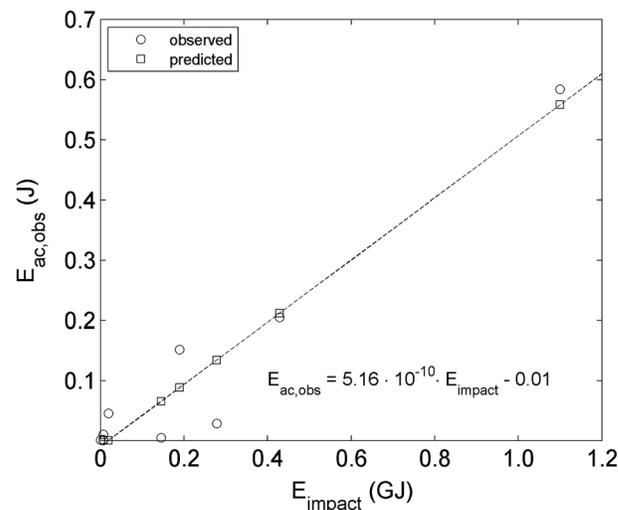
**Figure 3.** Relationship between the energy of block-water impact and both observed and predicted acoustic emissions. The coefficient of determination reached a value of 0.93. A low-pass Butterworth zero-phase filter with 200 Hz cutoff frequency was applied to the data before this analysis.
