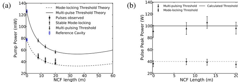
Fig. 3. (a) Predicted mode-locked ranges based on the measured reference cavity with experimental results. (b) Calculated peak pulse power corresponding to  $\phi_{max} = \pi$  with measured intra-cavity pulse peak powers at lower and higher points of fundamental mode-locking.
