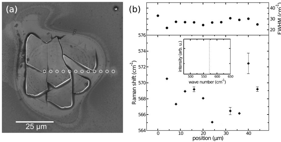
FIG. 1. (a) Scanning electron micrograph showing the ZnO surface after the modification by a single ultrashort laser pulse with a peak fluence of  $9 \text{ J/cm}^2$ . The white circles illustrate the points where Raman spectra were recorded. (b) Line widths (top) and center positions (bottom) of the  $A_1(\text{LO})$  phonon modes as obtained from the Raman scattered signal at the positions marked in (a). The inset shows Raman spectra measured at the position marked in red and blue.
