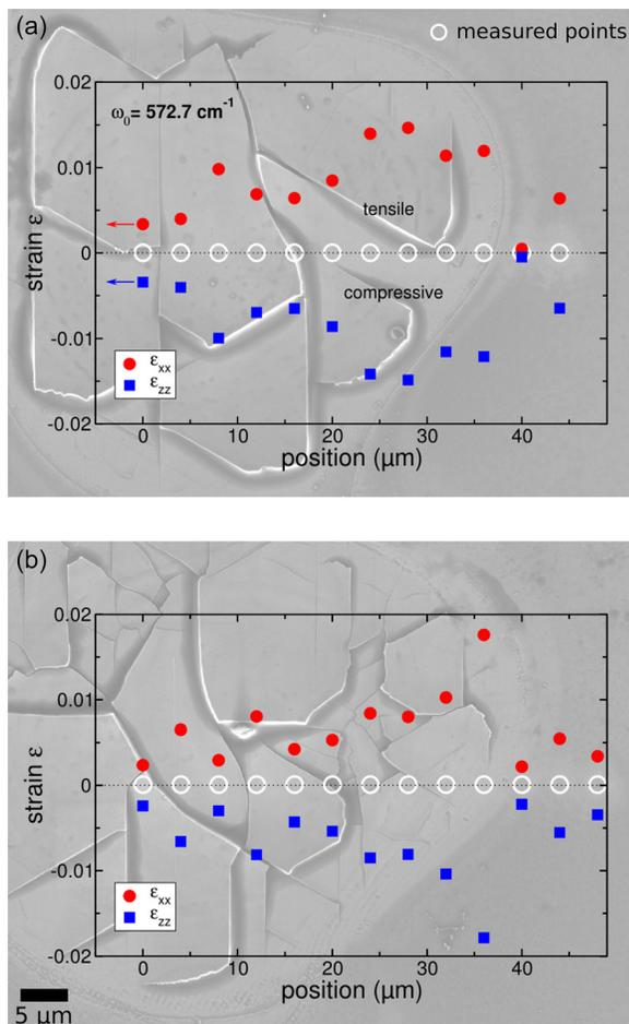
FIG. 2. In-plane  $\epsilon_{xx}$  and out-of-plane components  $\epsilon_{zz}$  of the strain tensor calculated from the Raman data at the positions of the measurements on the samples. Shown is the morphology and the strain after (a) one ultrashort pulse and (b) two ultrashort pulses with a peak fluence of  $9 \text{ J/cm}^2$ .
