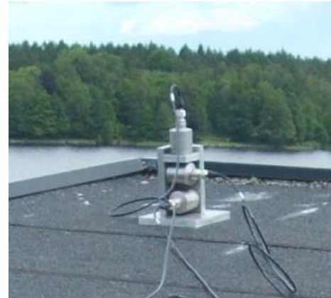
Figure 5: Accelerometers mounted to measure along three axes at a single point.
