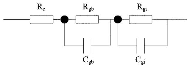
Figure 4 Equivalent circuit for frequency response of composite.
