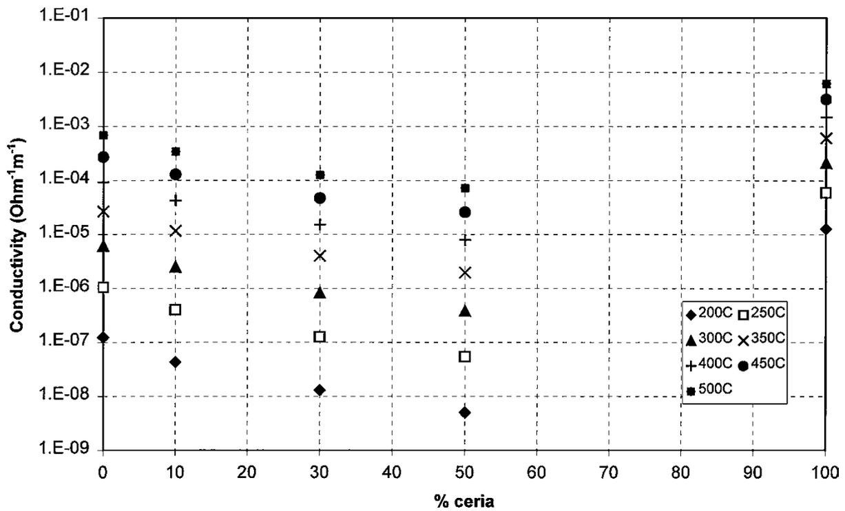
Figure 6 Conductivity versus percentage ceria in samples.
