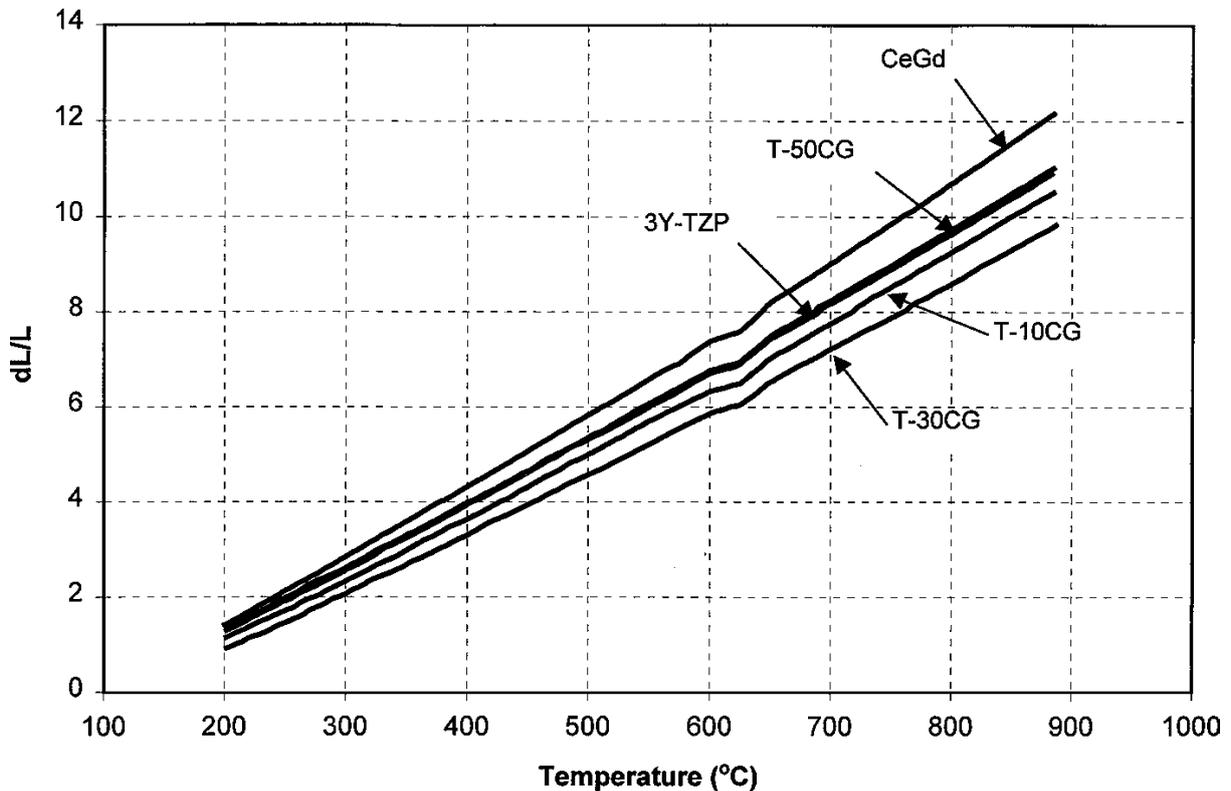
Figure 1 Thermal expansion ( $dL/L$ ) versus temperature.
