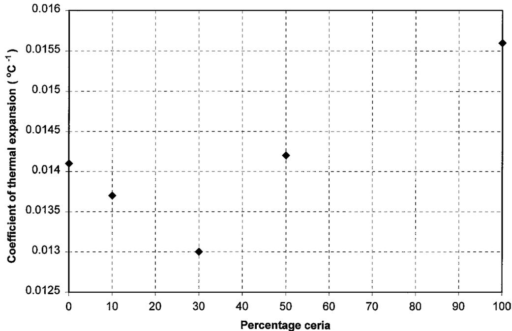
Figure 2 Coefficient of thermal expansion versus percentage ceria.
