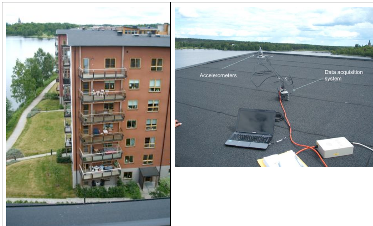
Figure 8: Limologen Building in Växjö, Sweden. Monitoring acceleration under ambient wind load
