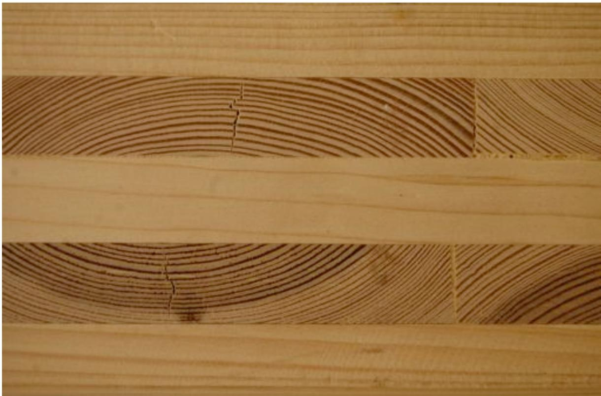
**Figure 3: Cross Laminated Timber (CLT)**
