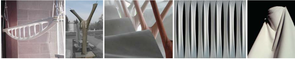
Figure 2. Fabric formwork (images courtesy Mark West, CAST).
