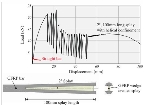
**Figure 4** – Splayed bar behaviour (after Darby et al., 2007).
