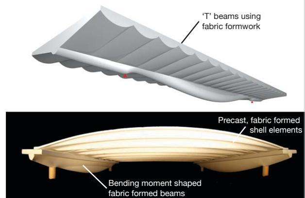
**Figure 5** – Long span fabric formed beams and shells.
