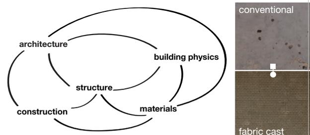
Figure 3 — Advantages (left) and improvements in surface quality when using fabric formwork (right).
