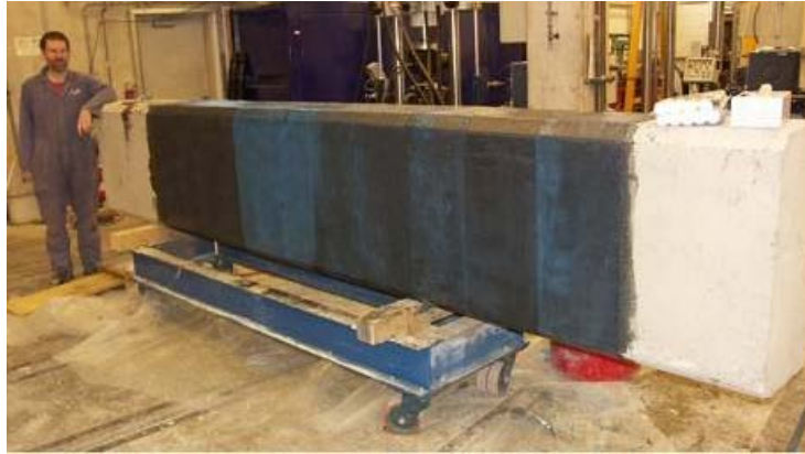
Figure 2: Fabric-wrapped shear specimen of realistic size
