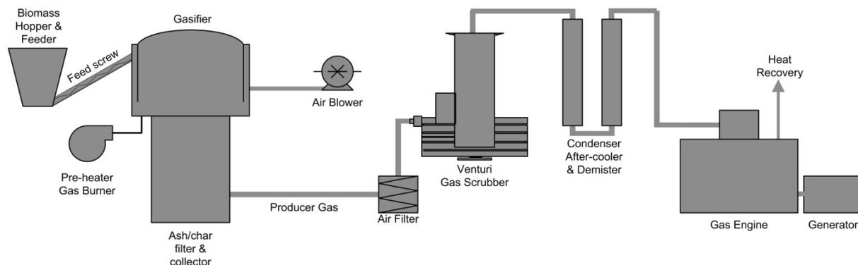
**Figure 1: Simplified Schematic of the Gasification Process**
