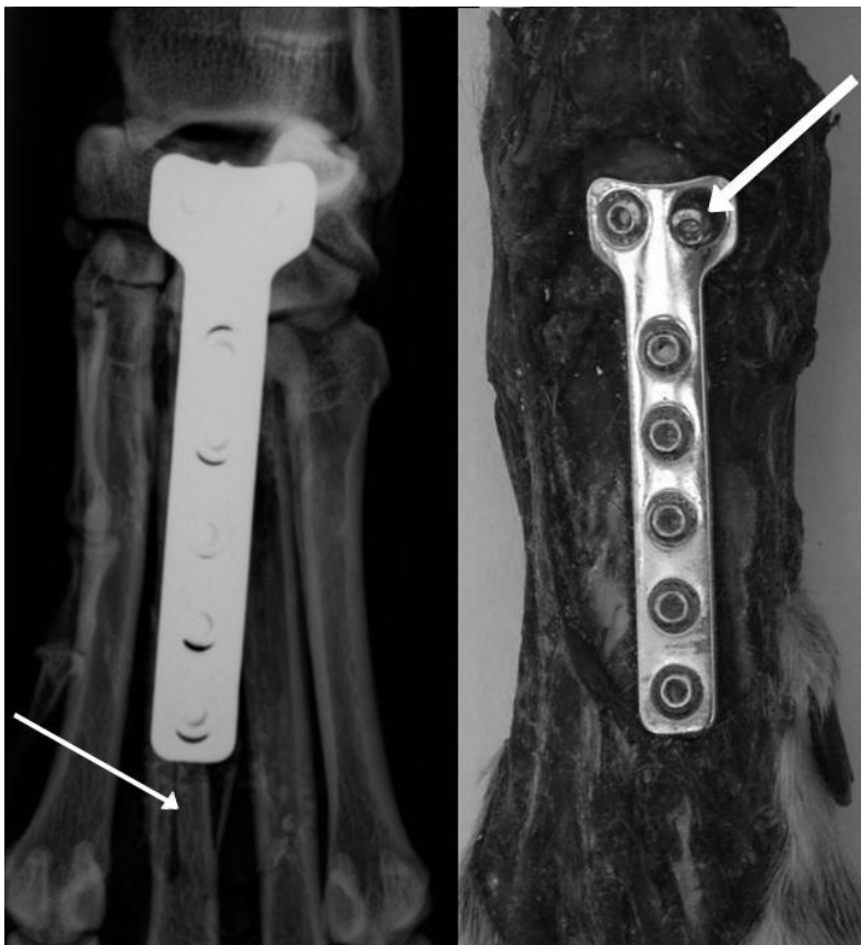
Figure 6: Radiograph (left) and photograph (right) of two of the T-plate constructs demonstrating metacarpal III fracture (thin white arrow) and loosening of a radial carpal bone screw (thick white arrow).
