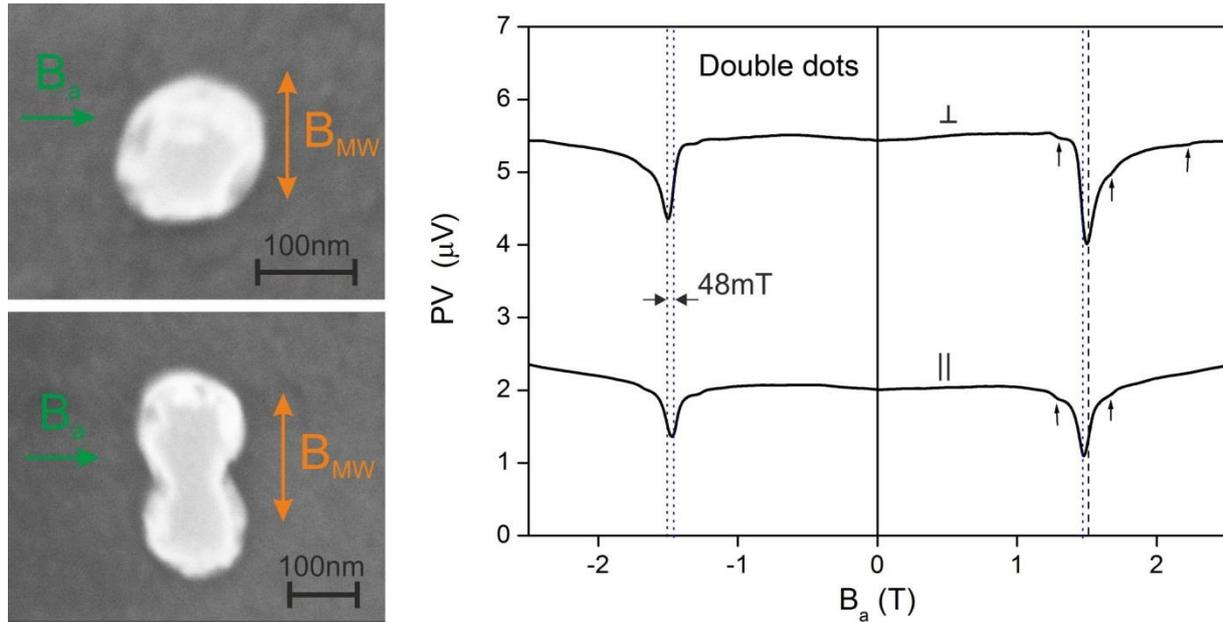
Fig. 5. (a) Dy dot and (b) overlapping dots. (c) Photovoltage spectroscopy of the overlapping dot when the microwave magnetic field is perpendicular to the plane of the 2DEG ( $\perp$ ) or along the long axis of the double dot ( $\parallel$ ).
