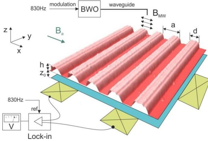
Fig. 1. Ferromagnetic finger gates fabricated on a GaAs/AlGaAs heterojunction. The fingers are magnetized by magnetic field  $B_a$  and irradiated by linearly polarized microwaves – magnetic field  $B_{MW}$  – supplied by a backward wave oscillator (BWO). Magnetic excitations are detected through the photovoltage they induce in the high mobility 2DEG.
