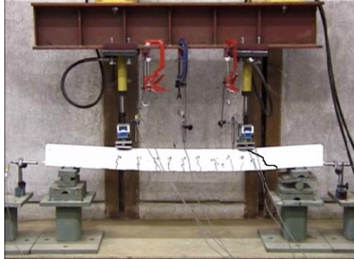
Figure 11. Beam test during size-effect series.
