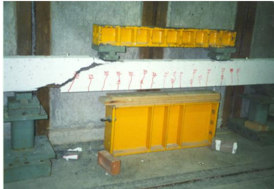
Figure 5. FRP deep-embedment shear-strengthened concrete beam.
