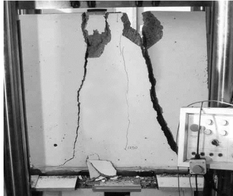
Figure 13. Interaction between multiple anchorages.
