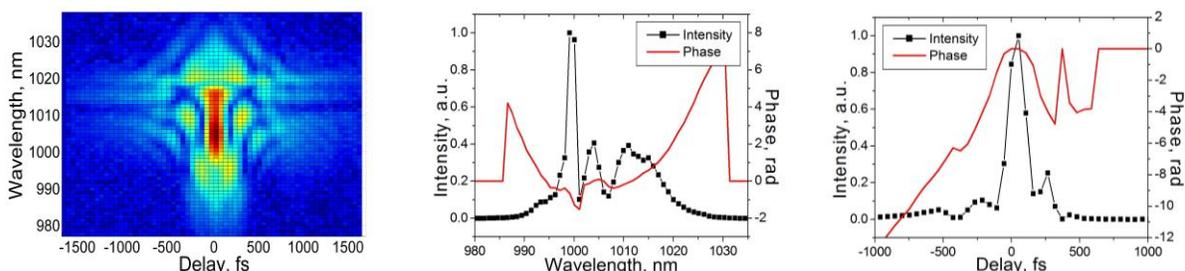
Figure 2. FROG spectrogram (a), and extracted spectral (b) and temporal characteristics (c) of the compressed output of the NKT fiber. A FWHM pulse duration of 150 fs is achieved at an average power of 270 mW.
