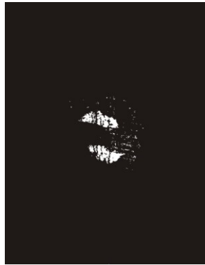
Figure 5 Image of the defect using ultrasonic C-Scan
