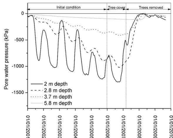
**Figure 4. Finite element calculations of pore water pressure for the crest of the north embankment slope**
