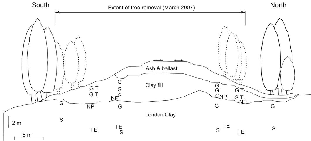
**Figure 1. A cross section of the instrumented embankment showing the location of Geo-piezometers (G), Standpipe piezometers (S), Inclometers (I), Extensometers (E), Neutron probe (NP) and TDR Theta probes (T).**
