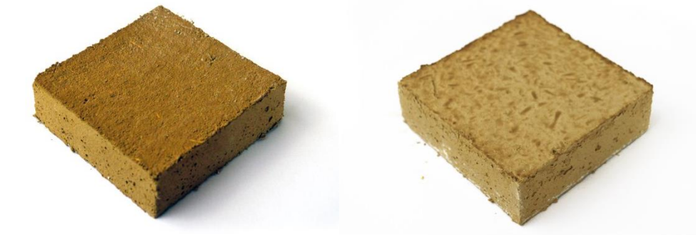
Figure 2. Novel clay coatings with pumice (left) and hemp (right) aggregates
