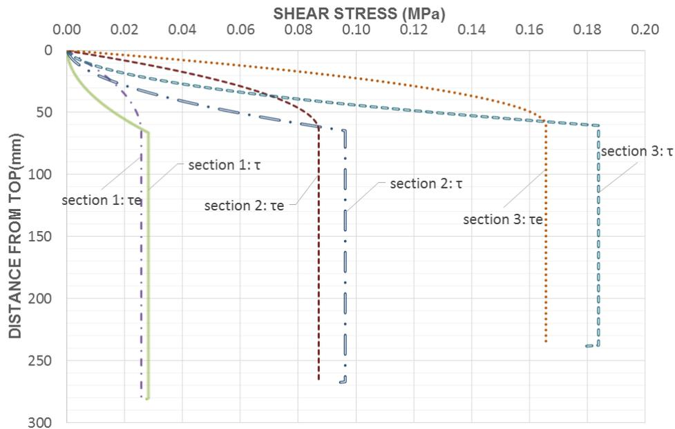
Figure 7: The shear stress distribution of sections
