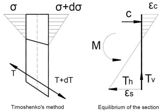
Figure 5: The bending stresses of the Timoshenko method
