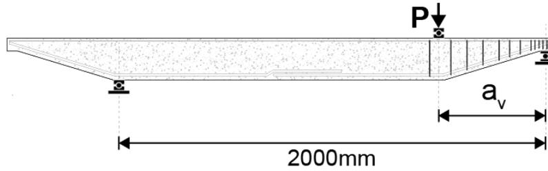
Figure 10: The test arrangement by Orr *et al.* [1]
