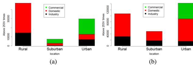
Figure 5 Location and customer mix of substation with voltage above 253V in high summer (a) and winter (b)
