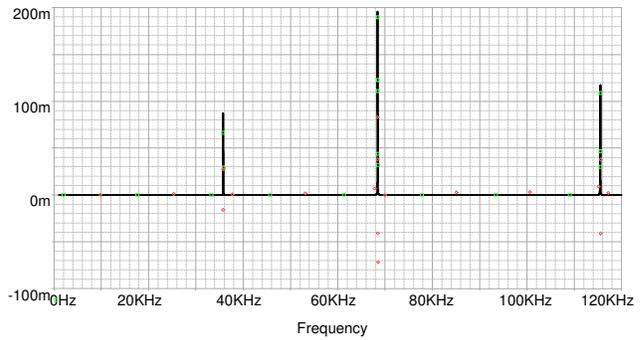
Fig.11 Real part of the admittance showing fundamental, 3<sup>rd</sup> and 5<sup>th</sup> harmonics of the transducer model.
