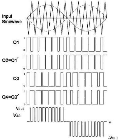
Fig.6 Generation of PWM, switching and output waveforms.
