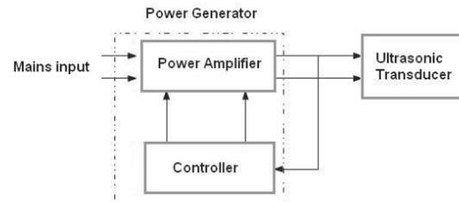
Fig.1 Typical layout of a power ultrasonic system.
