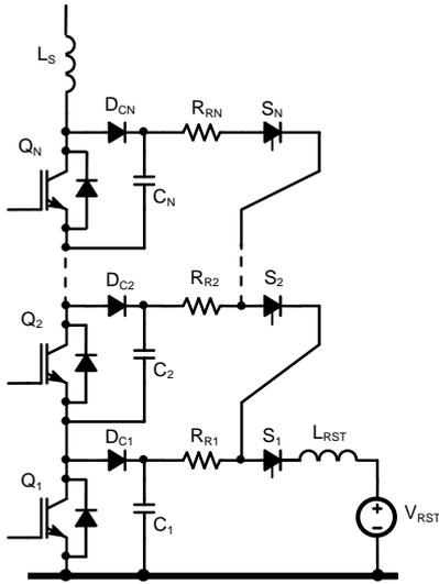
Figure 4: Series RCD scheme with reset switches.
