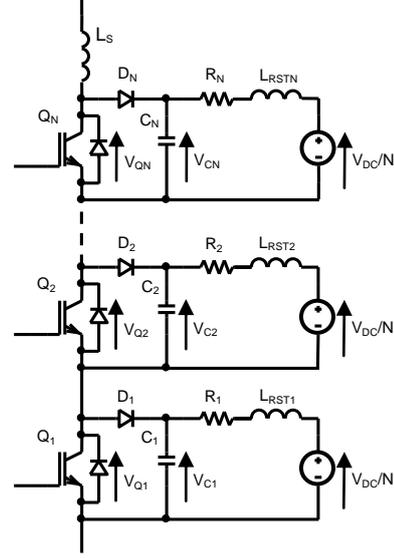
Figure 3: Impractical RCD scheme for series devices.
