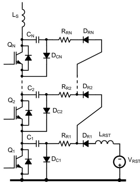
Figure 6: Series RCD scheme without switches.
