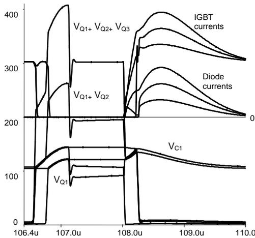
Figure 8: Asymmetric switching waveforms for Figure 6.
