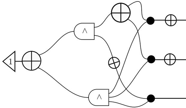
FIG. 20. Naïve CTNS realization of the familiar W-state  $|001\rangle + |010\rangle + |100\rangle$ . A standard (temporal) acyclic classical circuit decomposition in terms of the XOR-algebra realizes the function  $f_W$  of three bits. This function is given a representation on tensors. As illustrated, the networks input is post selected to  $|1\rangle$  to realize the desired W-state.
