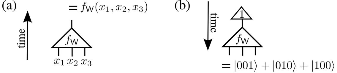
FIG. 19. Left (a) the circuit realization (internal to the triangle) of the function  $f_W$  of e.g. (23) which outputs logical-one given input  $|x_1x_2x_3\rangle = |001\rangle$ ,  $|010\rangle$  and  $|100\rangle$  and logical-zero otherwise. Right (b) reversing time and setting the output to  $|1\rangle$  (e.g. post-selection) gives a network representing the W-state. The naïve realization of  $f_W$  is given in Figure 21 with an optimized co-algebraic construction shown in Figure 21.
