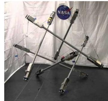
Fig. 4. NASA ‘Superball’ tensegrity robot platform [12,13]
