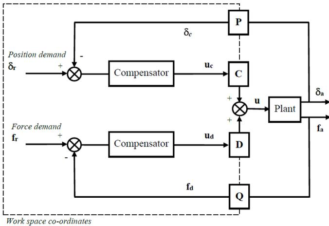
Fig. 11 Multi-axis control scheme (modified from [14])
