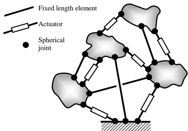
Fig.1. Example PKM schematic with multiple bodies (nodes)
