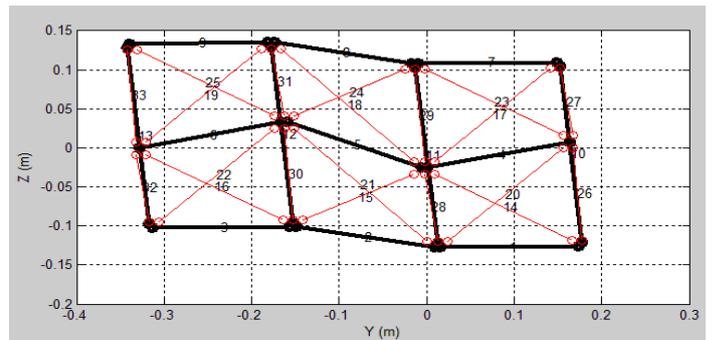
Fig. 10. Shear displacement (contracting 15 and 24, extending 18 and 21)
