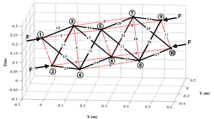
Fig. 6. Example tensegrity structure (struts are thick lines)
