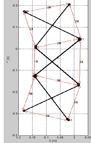
Fig. 9. Bending displacement (contracting 15 and 18, extending 21 and 24)
