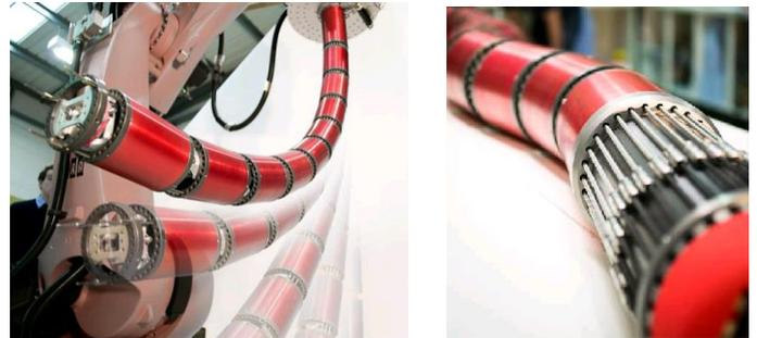
Fig.5 The first commercial snake arm robot (www.ocrobotics.com)
