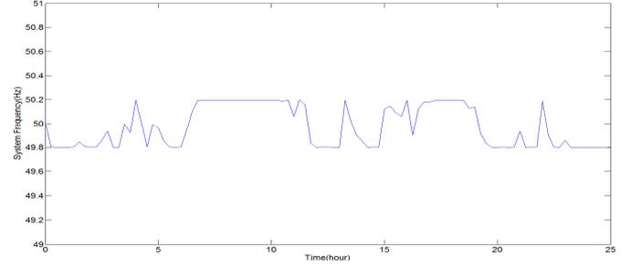
Fig. 7. System frequency with the correction of frequency regulation based on 30-minute rolling average load in day 1
