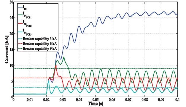
Figure 3. Fault currents for different SFCL effective parameters.
