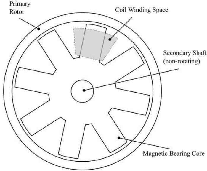
**Figure 2.** Schematic cross-section of internal magnetic bearing
