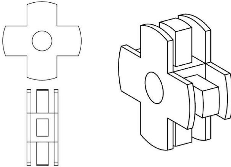
**Figure 11.** An internal-stator homopolar bearing core design
