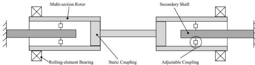
**Figure 9.** Schematic of novel rotor test rig
