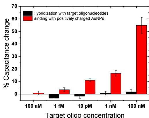
Fig. 3. Dose response. Black bars represent changes in capacitance on binding with target oligo while red bars represent amplification in capacitance change on binding with AuNPs.
