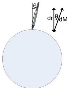
Figure 3 – Probe Cosine Error
