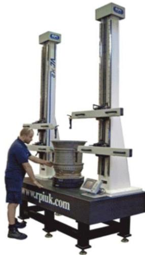
Figure 2 – An Axi-Symmetric Measurement Machine
