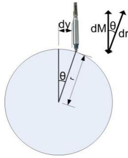
Figure 4 – Probe Off-Centre Error
