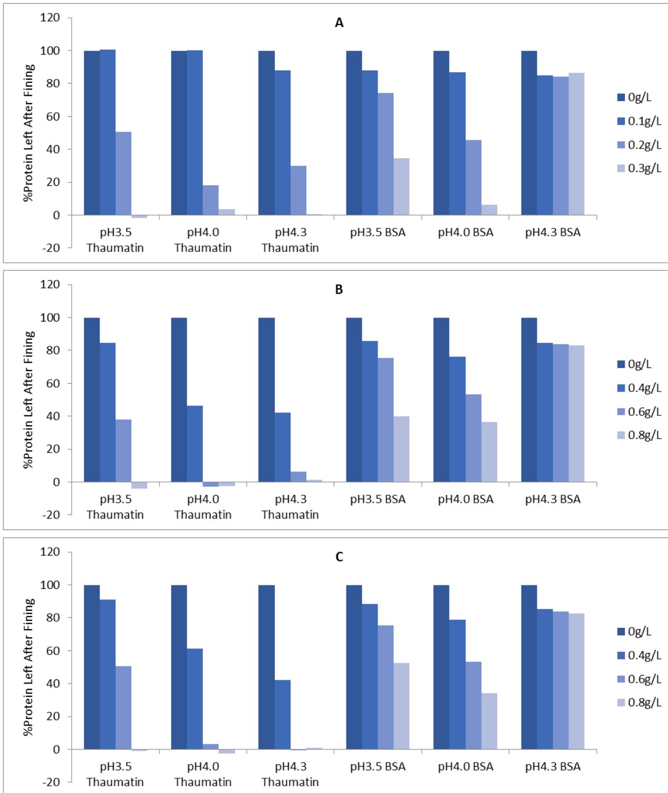
Figure 2: Fining test results on model wine solutions at various pH. A: Bentonite A concentration at 0.1, 0.2 and 0.3g/L; B: Bentonite B concentration at 0.4, 0.6, 0.8g/L; C: Bentonite C concentration at 0.4, 0.6, 0.8g/L.
