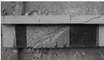
SC0.7U ( \beta = 35^\circ , V_u = 166 kN)
