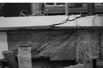
LB1.3UA ( \beta = 37^\circ , V_u = 511 kN)
