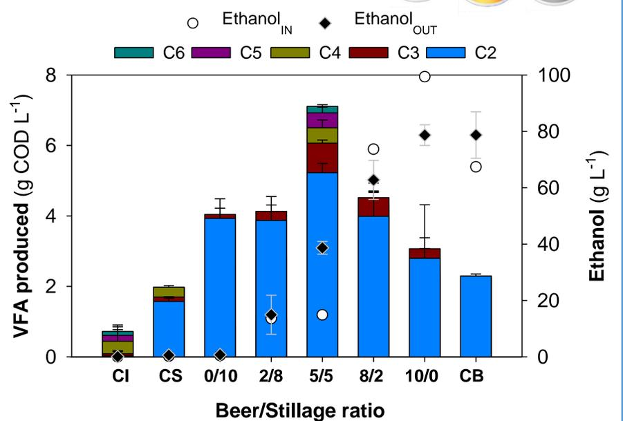
Figure 4. Produced VFA and ethanol concentration with different stillage & beer ratios. (CI, CS, CB stand for controls with only inoculum, stillage or beer, respectively).
