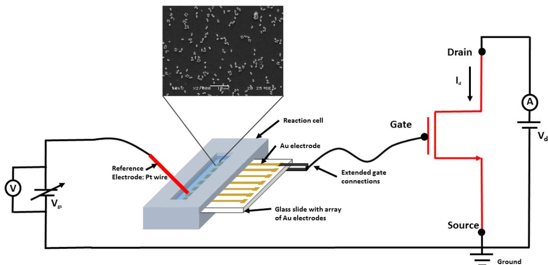
Figure 1 - Working principle of the BioFET sensor. An array of evaporated gold electrodes placed in a flow cell is connected to the gate of a MOSFET. An external reference electrode is used to apply the gate voltage. The same electrodes were used for EIS and MALDI-ToF measurements.
