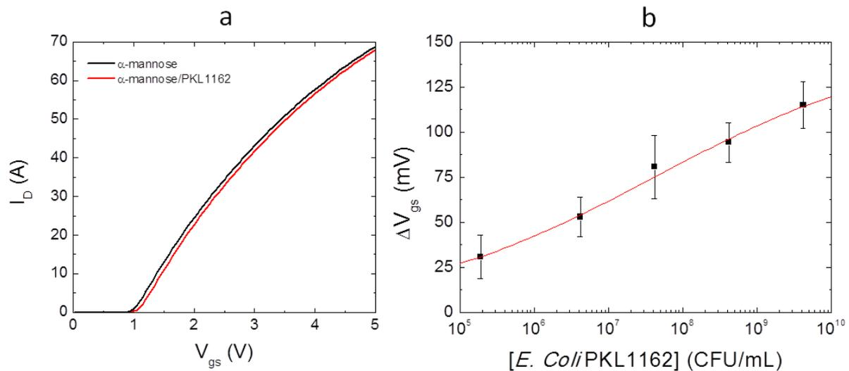
Figure 3 - Bacterial detection using BioFETs. a) BioFET  $I_D/V_{gs}$  characteristic for an electrode before (black line) and after (red line) *Escherichia coli* binding. b)  $V_{gs}$  changes vs. bacterial concentration. The line represents a fit to the data with a Hill-type response ( $R^2 = 0.990$ ).
