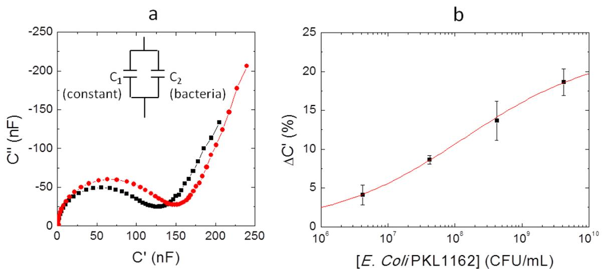
Figure 2 - Bacterial detection performing EIS capacitive measurements. a) Complex capacitance Cole-Cole plots for an electrode before (black line, squares) and after (red line, circles) *Escherichia coli* PKL1162 binding. The inset shows a schematic equivalent circuit.
