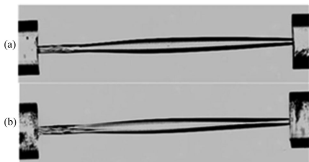
Fig. 7. 600 \mu\text{m} bridges associated with two different eosin concentration samples showed in Fig. 6. For photopolymerization, light was incident from the right-hand fiber. (a) 0.5 wt.%, (b) 0.2 wt.%.
